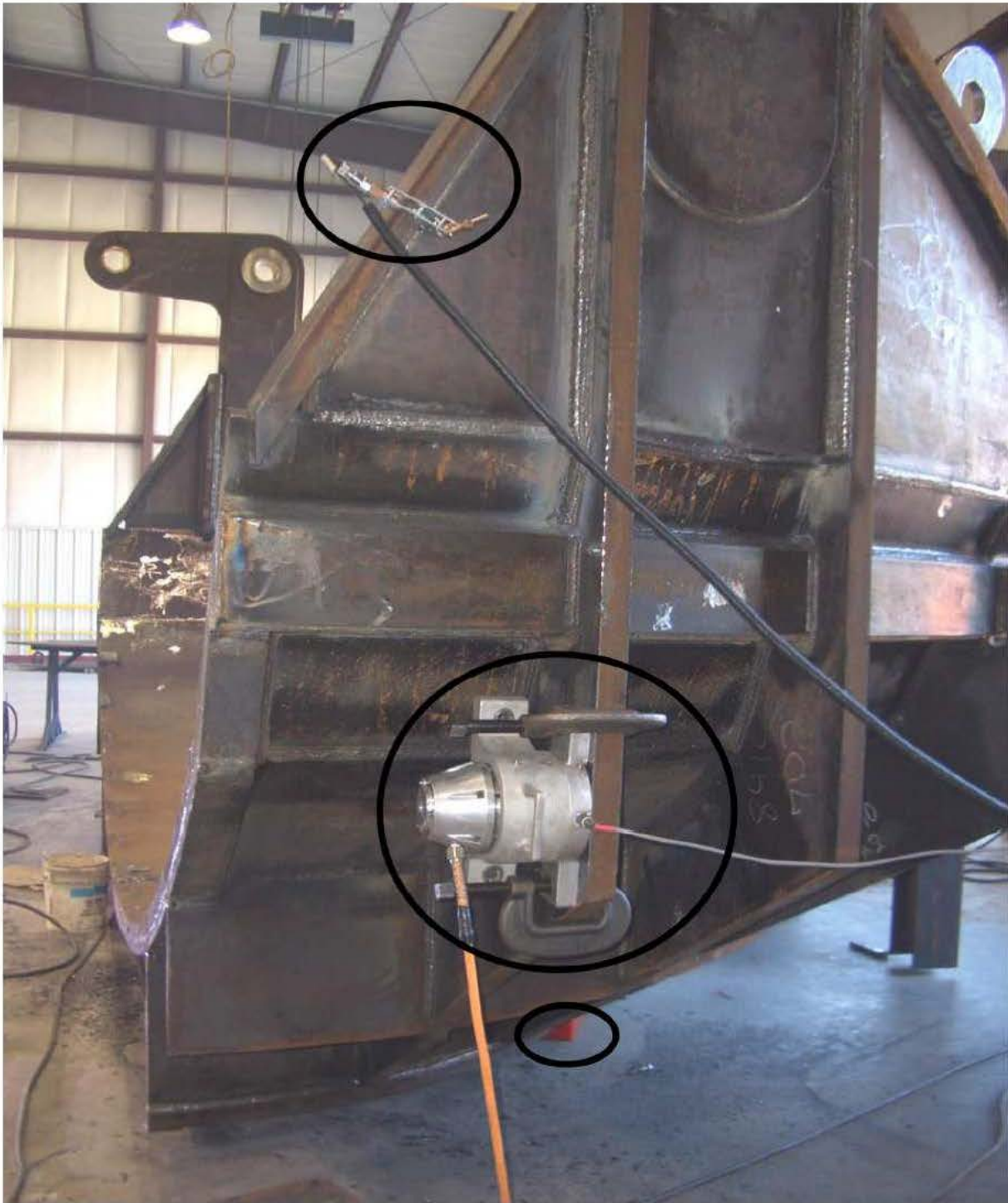
Figure 2: Another view of Clamshell setup for VSR Treatment. One of two Load Cushions supporting the rear of the Clamshell is visible (circled), below the Vibrator (circled). Note that the support leg on the right is purposely not touching the floor; the full weight of the workpiece rested on the 4 Load Cushions.
