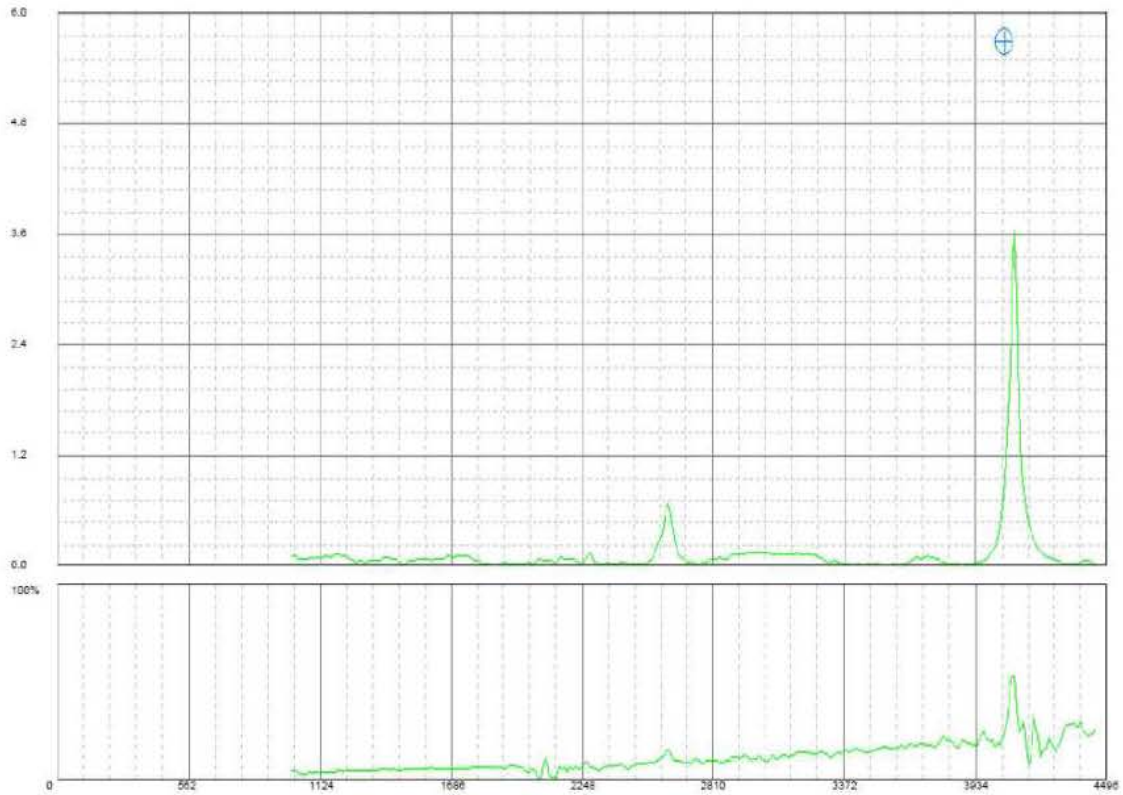
Figure 3: First Pre-Treatment Scan. VSR Treatment Charts consist of two plots: An upper plot of workpiece acceleration and a lower plot of vibrator input power, both of these plotted on a vertical axis vs. a common horizontal axis of vibrator RPM. Peaks in the upper plot are resonances of the workpiece. Peaks in the lower plot are resonances that cause increased, perhaps excessive, vibrator input power (excessive power is easily rectified by lowering the Vibrator unbalance setting, repositioning the Vibrator, or a combination of both).
