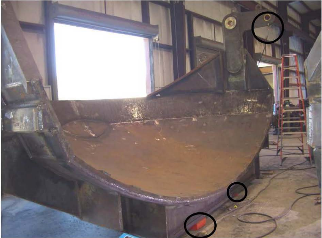
Figure 1: 24.5 ton Clamshell Bucket half setup for VSR Treatment. Note location of two Load Cushions (circled); the other two Cushions were placed on the opposite side (one being visible in Figure 2). The Accelerometer is visible on right lifting arm (circled), near the top of the photo. This particular Accelerometer location was used during a second Treatment of this workpiece, which turned out to be unnecessary (first VSR Treatment was fully effective), as indicated by the VSR Treatment Charts shown in Figures 3 – 6.
